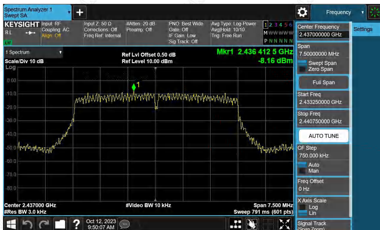
Figure 8: Power Spectral Density, Bandwidth 5MHz, 2437MHz
