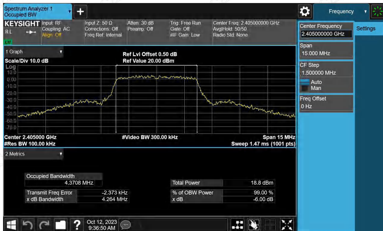
Figure 1: 6dB Bandwidth, Bandwidth 5MHz, 2405MHz
