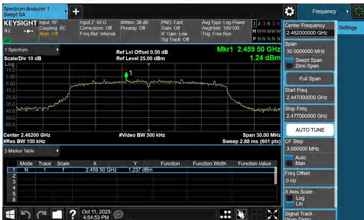
Figure 18: Conducted Spurious Emission & Authorized-band band-edge, 2462MHz, Bandwidth 20MHz Carrier Level
