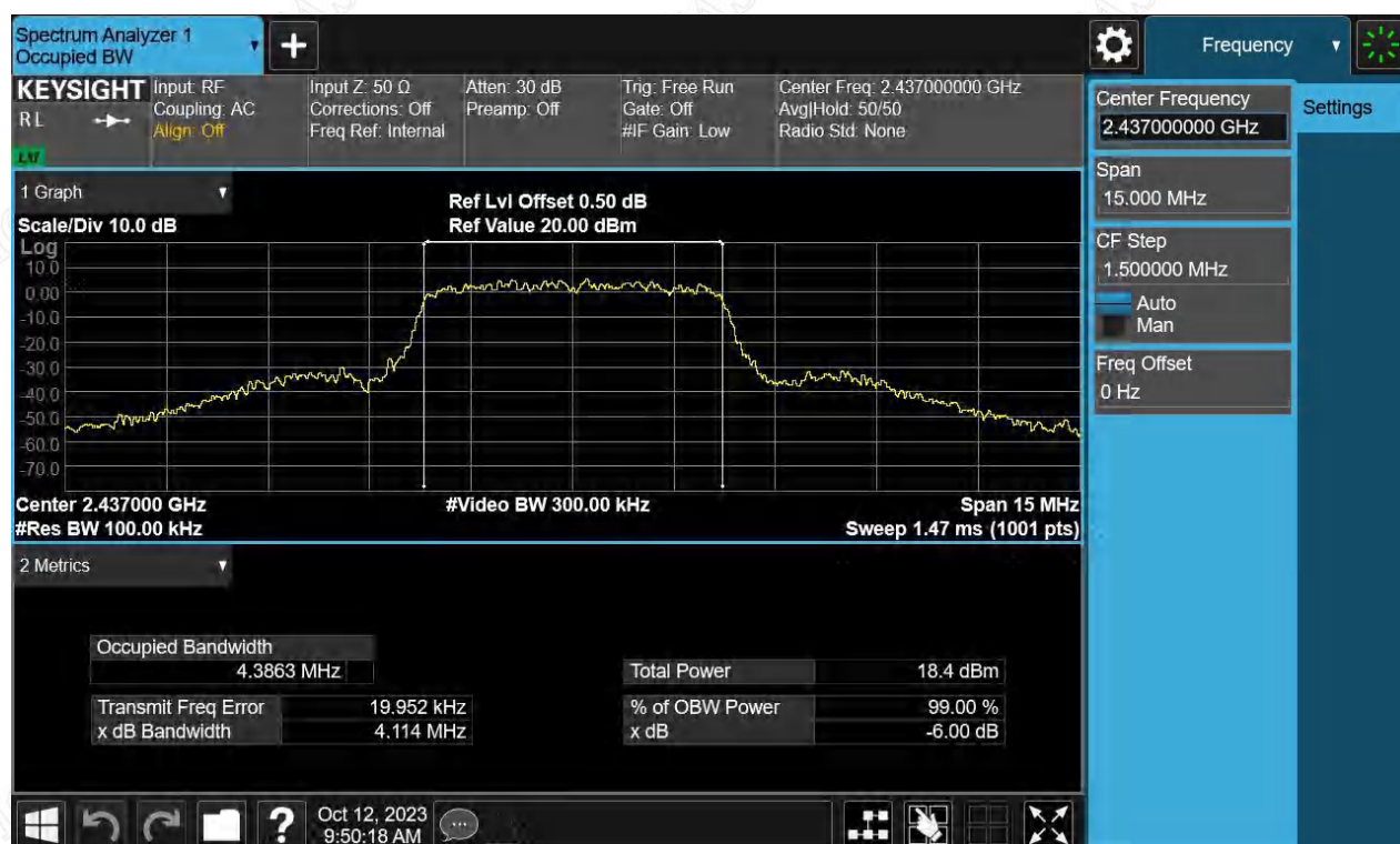
Figure 2: 6dB Bandwidth, Bandwidth 5MHz, 2437MHz
