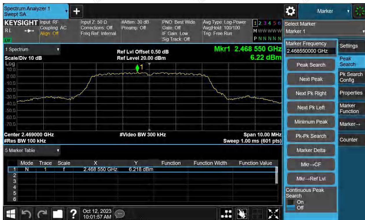
Figure 15: Conducted Spurious Emission & Authorized-band band-edge, 2469MHz, Bandwidth 5MHz Carrier Level
