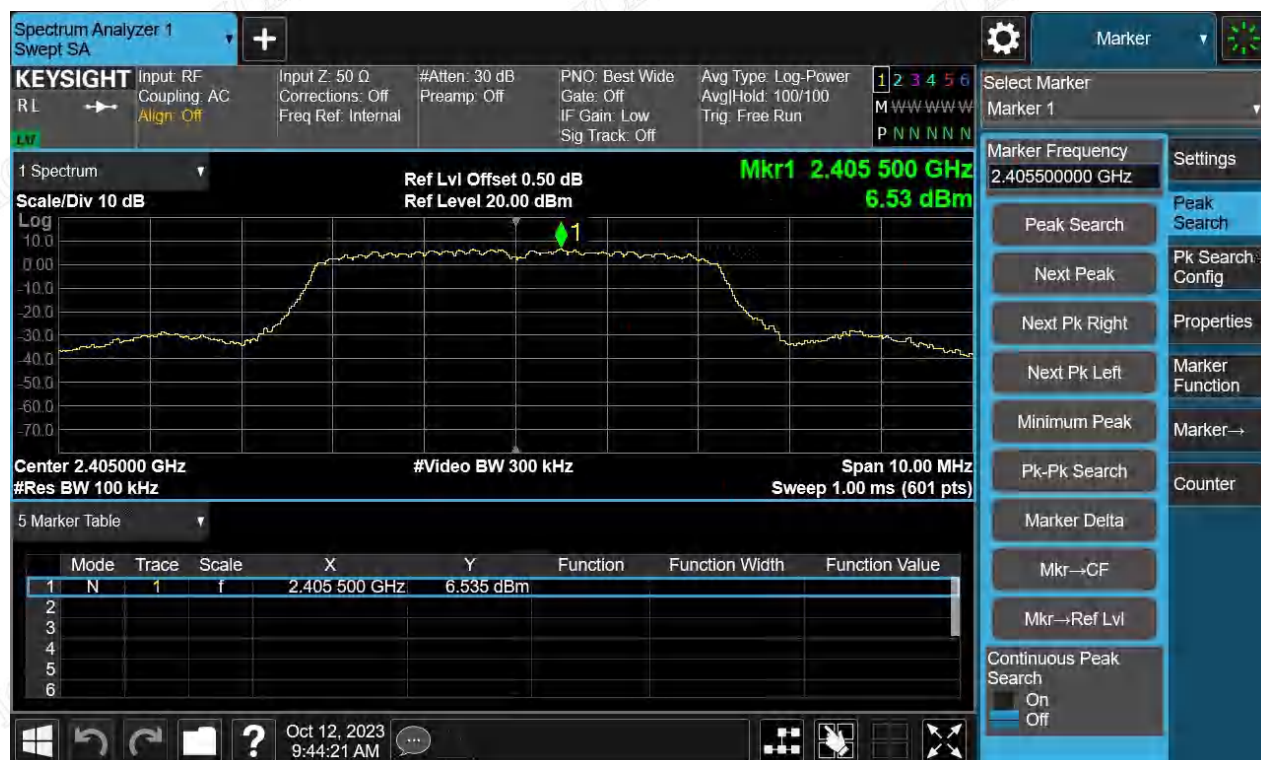
Figure 13: Conducted Spurious Emission & Authorized-band band-edge, 2405MHz, Bandwidth 5MHz Carrier Level
