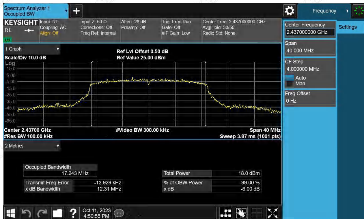
Figure 5: 6dB Bandwidth, Bandwidth 20MHz, 2437MHz
