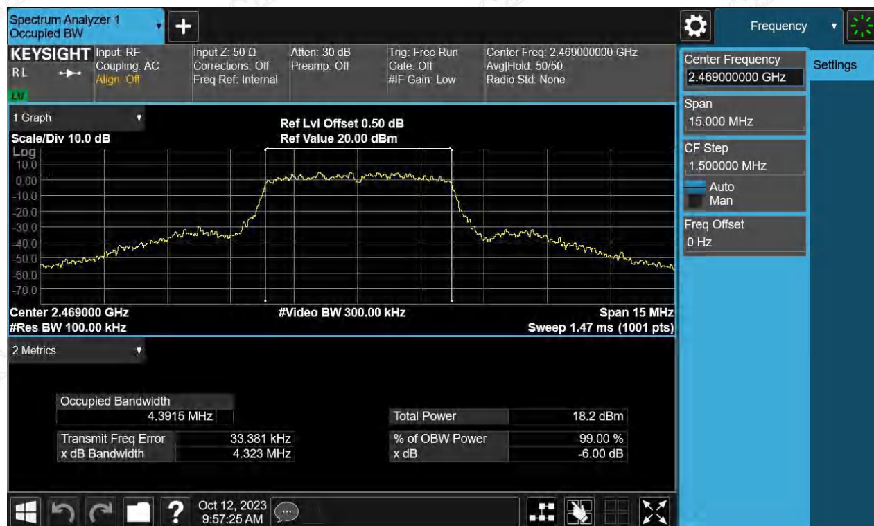
Figure 3: 6dB Bandwidth, Bandwidth 5MHz, 2469MHz
