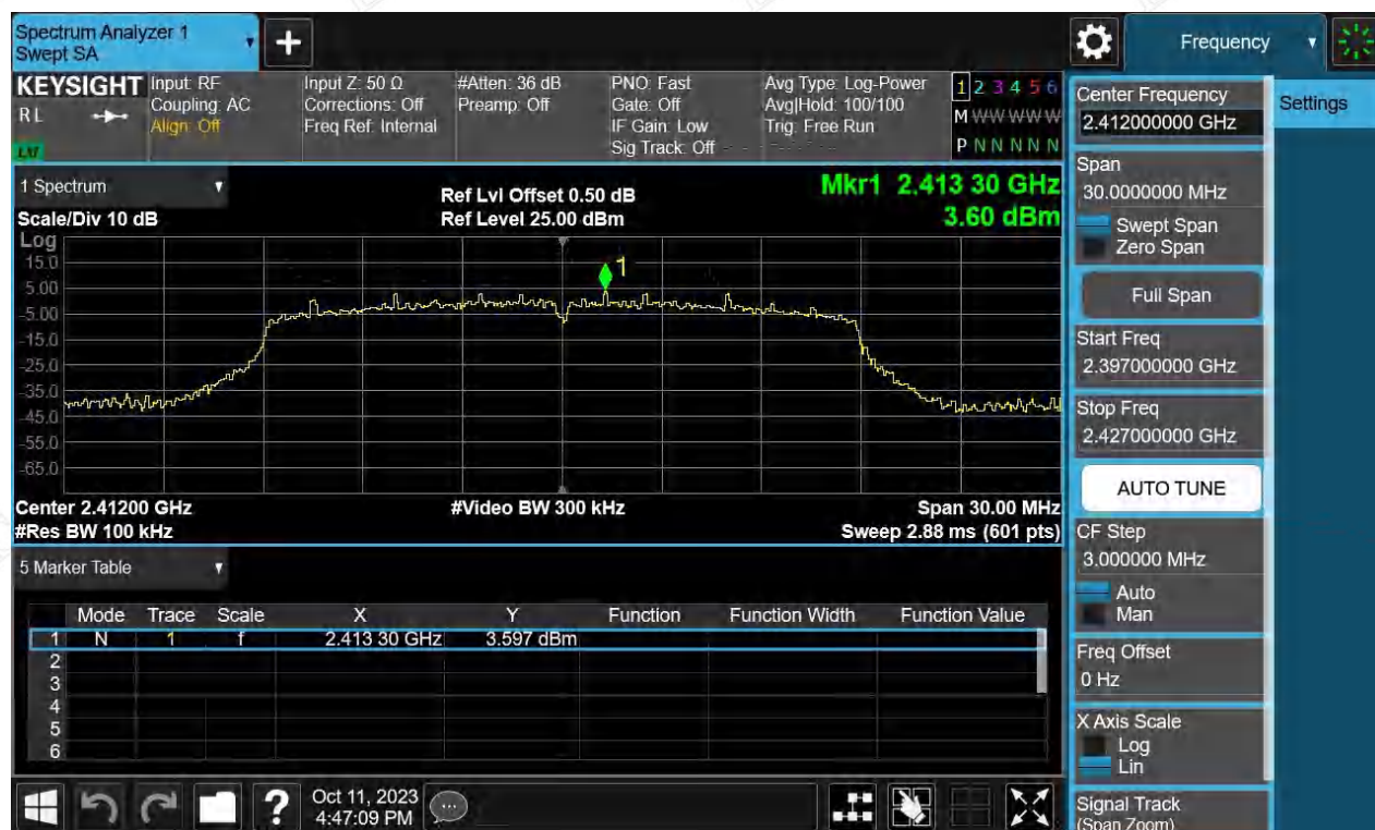
Figure 16: Conducted Spurious Emission & Authorized-band band-edge, 2412MHz, Bandwidth 20MHz Carrier Level
