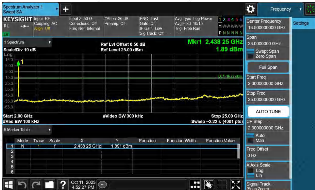
Figure 18: Conducted Spurious Emission & Authorized-band band-edge, 2462MHz, Bandwidth 20MHz Carrier Level
