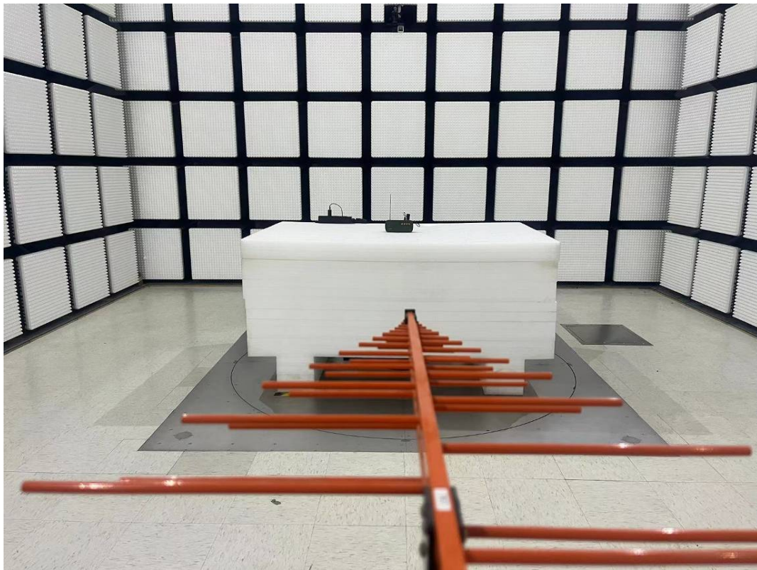
Radiated Emission Above 1GHz View
