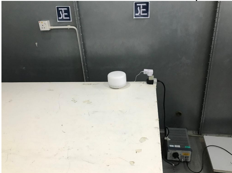
Measurement of Conducted Emission Test Set Up
