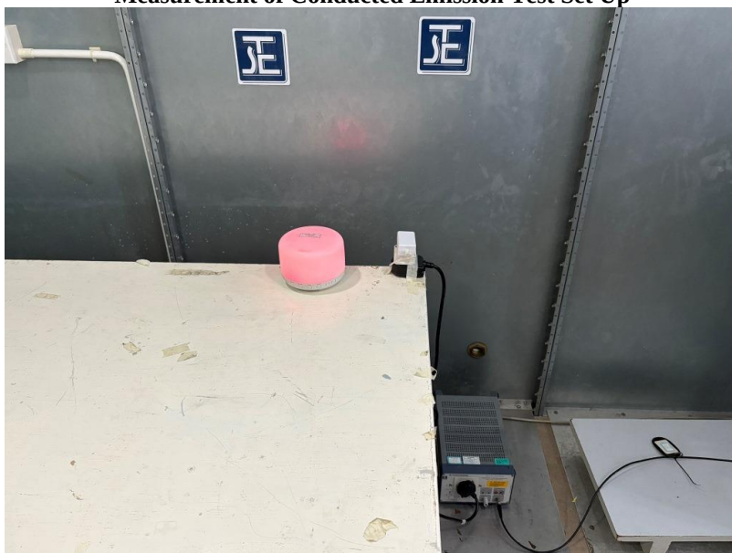
Measurement of Conducted Emission Test Set Up
