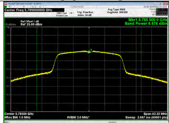
Conducted AVG output power IEEE 802.11ac_20_Channel 157_Antenna 0
