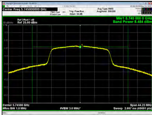
Conducted AVG output power IEEE 802.11a_Channel 149_Antenna 0
