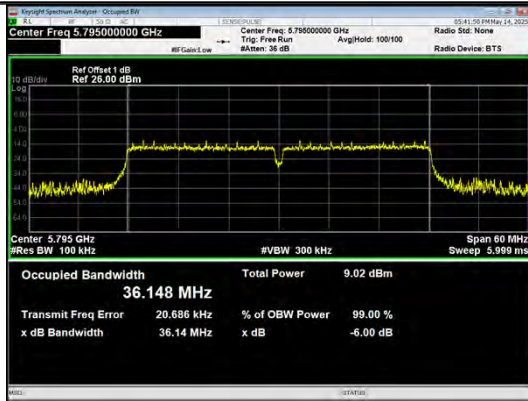
IEEE 802.11ac_Channel 159_40MHz_Antenna 0
