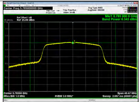
Conducted AVG output power IEEE 802.11a_Channel 157_Antenna 0
