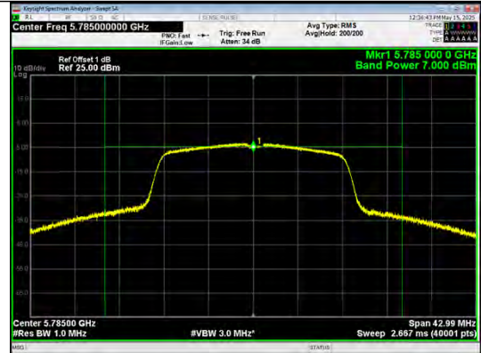
Conducted AVG output power IEEE 802.11ac_20_Channel 157_Antenna 0
