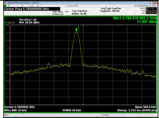
NT/NV_Antenna 0 IEEE 802.11ac_Channel 157_20MHz
