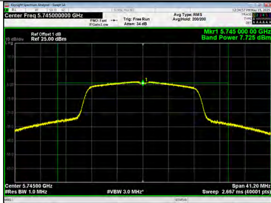
Conducted AVG output power IEEE 802.11ac_20_Channel 149_Antenna 0
