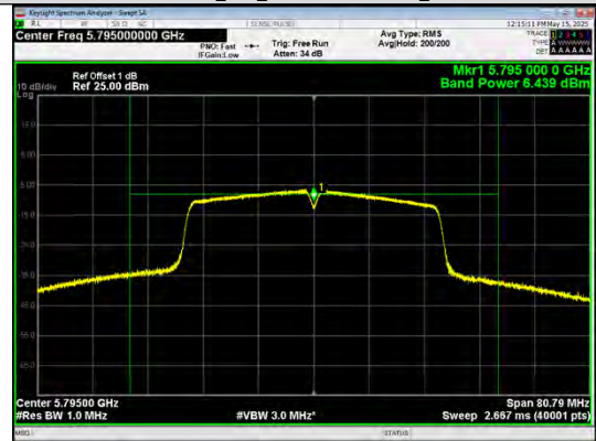
Conducted AVG output power IEEE 802.11n_40_Channel 159_Antenna 0
