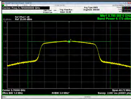
Conducted AVG output power IEEE 802.11n_20_Channel 157_Antenna 0
