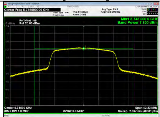
Conducted AVG output power IEEE 802.11n_20_Channel 149_Antenna 0
