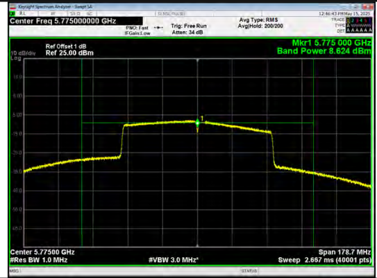
Conducted AVG output power IEEE 802.11ac_80_Channel 155_Antenna 0
