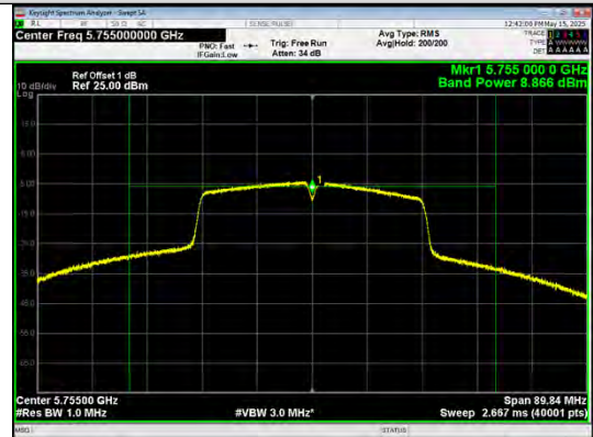
Conducted AVG output power IEEE 802.11ac_40_Channel 151_Antenna 0
