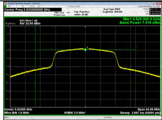
Conducted AVG output power IEEE 802.11n_20_Channel 165_Antenna 0
