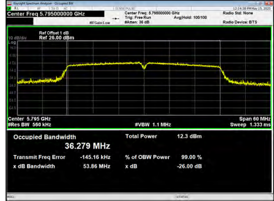
IEEE 802.11n_Channel 159_40MHz_Antenna 0
