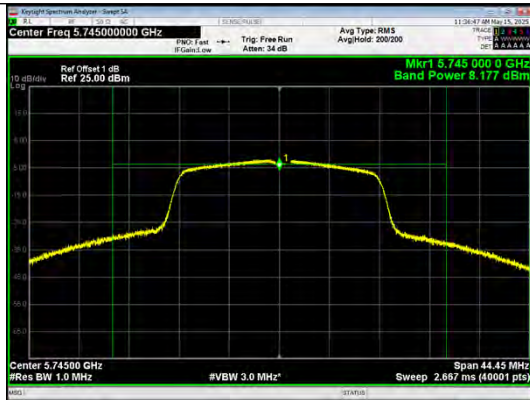
Conducted AVG output power IEEE 802.11a_Channel 149_Antenna 0
