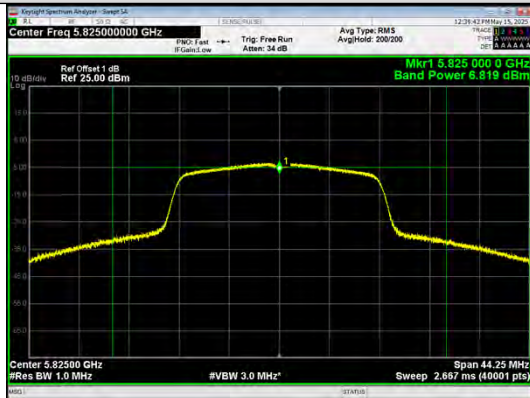
Conducted AVG output power IEEE 802.11ac_20_Channel 165_Antenna 0
