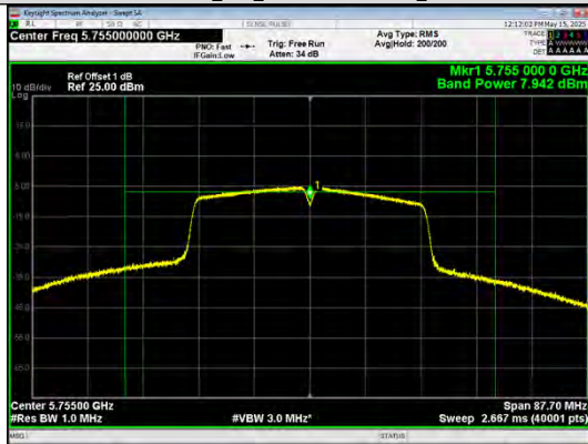
Conducted AVG output power IEEE 802.11n_40_Channel 151_Antenna 0
