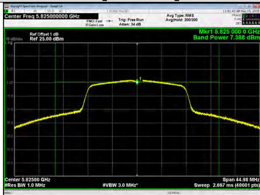
Conducted AVG output power IEEE 802.11a_Channel 165_Antenna 0
