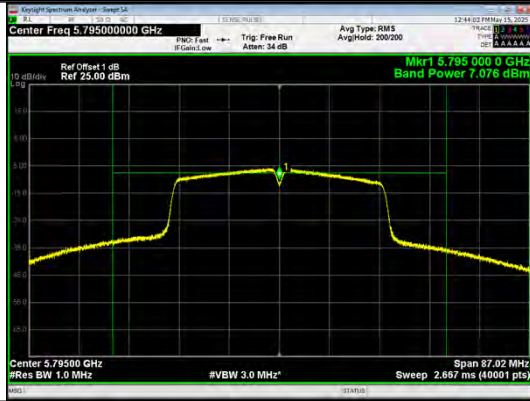
Conducted AVG output power IEEE 802.11ac_40_Channel 159_Antenna 0
