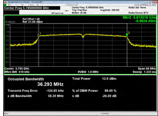
IEEE 802.11n_Channel 159_40MHz_Antenna 0
