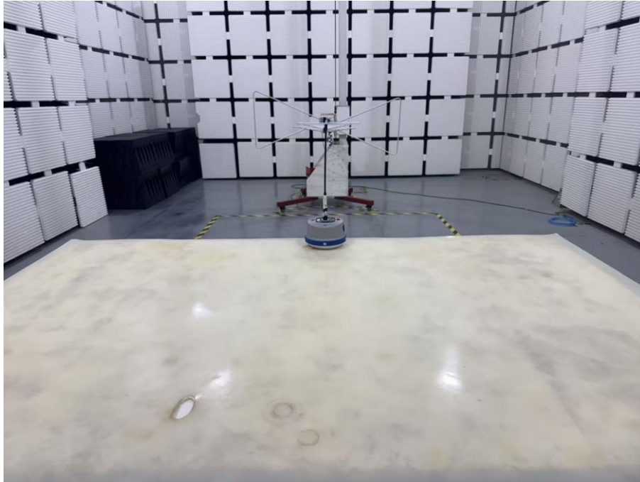
Set-up for Radiated Spurious Emission, Above 1GHz
