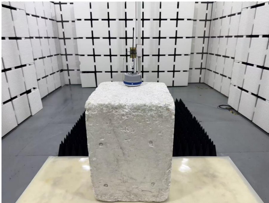
Set-up for Radiated Spurious Emission, Above 1GHz
