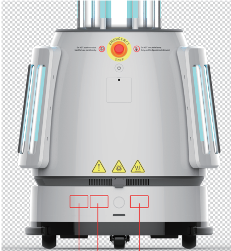
Fuselage Sticker Serial number collection sticker for the whole machine & access control plate FCC Sticker
