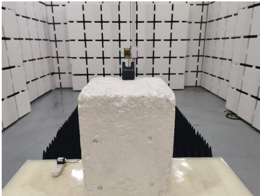
Set-up for Radiated Spurious Emission, Above 1GHz
