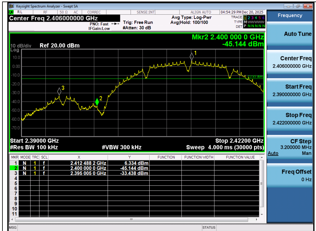
Test_Graph_802.11b_ANT1_2412_1Mbps_Lower Band Edge Emissions
