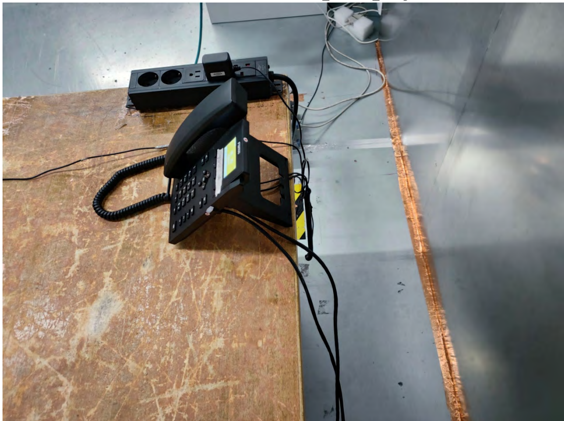
Conducted Emissions - Side View_X301W_Adapter 2
