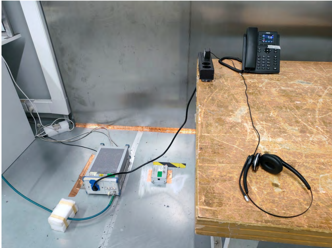
Conducted Emissions - Front View_J303W_Adapter 2
