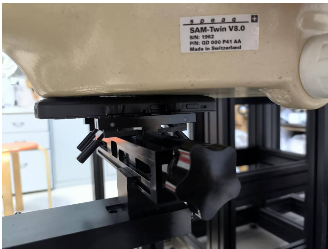
Body Back Setup Photo (0 mm)
