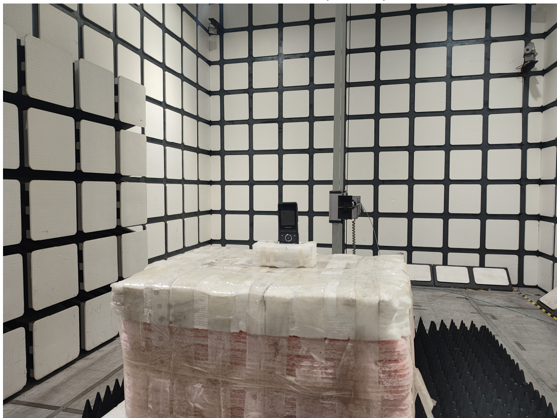
Radiated Emissions View (18-25 GHz)
