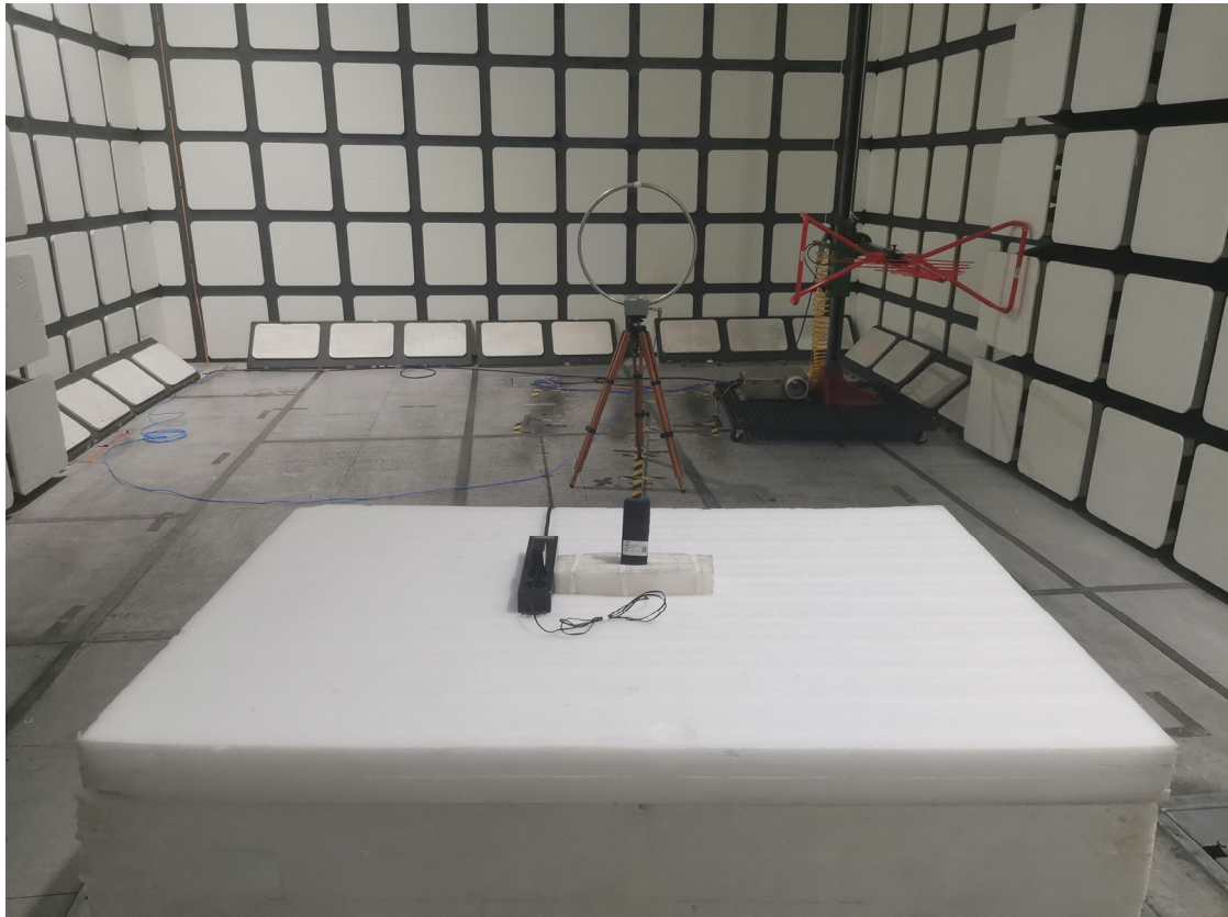
Radiated Emissions View (Below 1 GHz)
