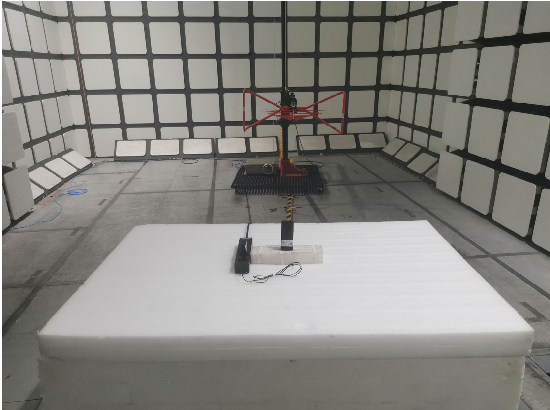
Radiated Emissions View (Below 1 GHz)
