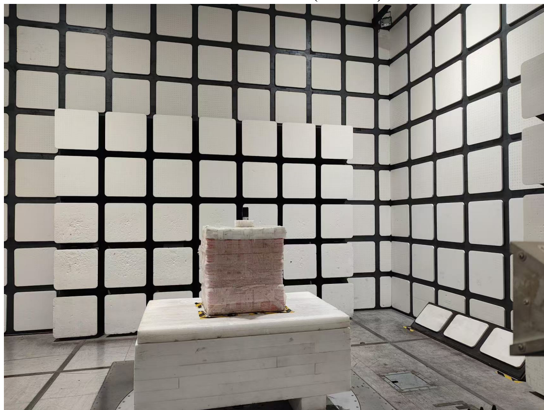
Radiated Emissions View (18-25 GHz)
