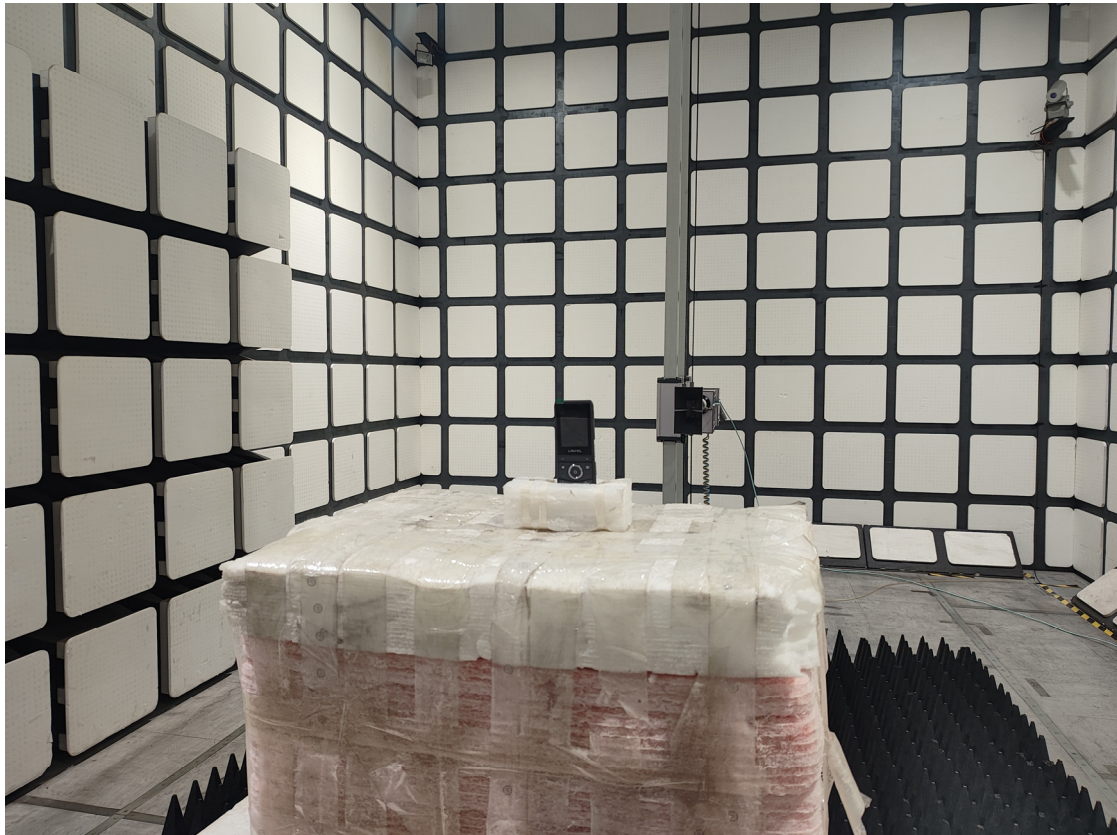
Radiated Emissions View (18-25 GHz)
