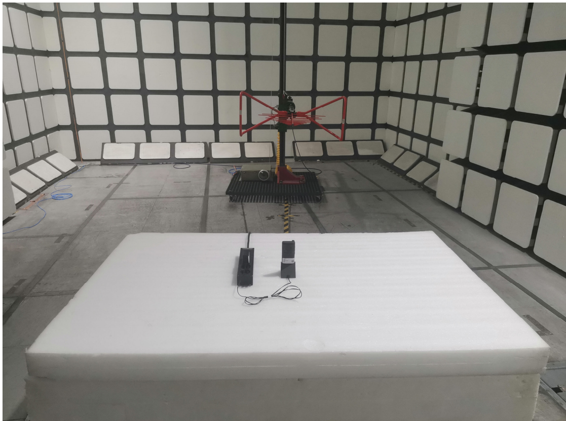
Radiated Emissions View (Below 1 GHz) (Charger)
