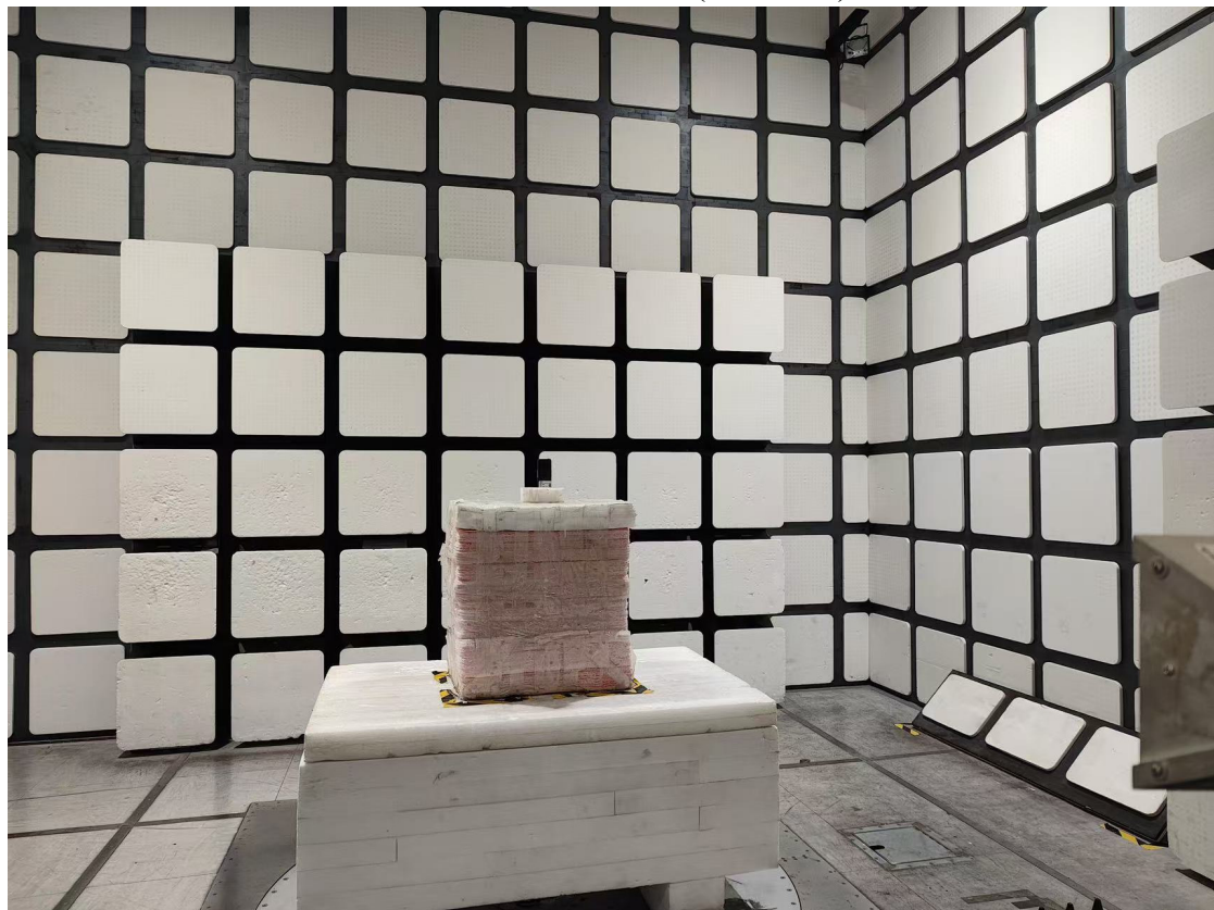
Radiated Emissions View (18-25 GHz)
