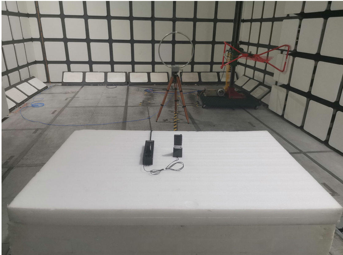
Radiated Emissions View (Below 1 GHz) (Charger)
