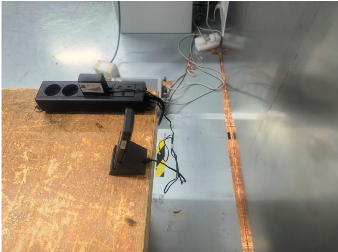
Conducted Emissions - Side View_ Adapter 1+Charger
