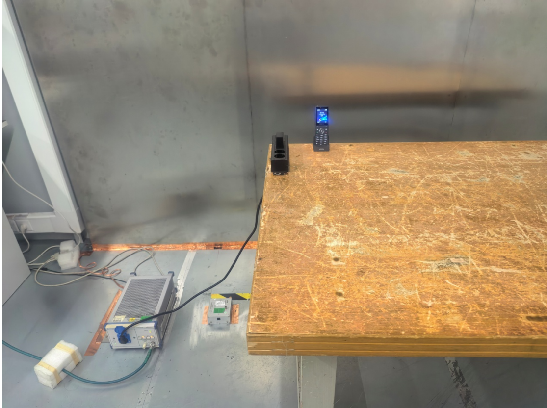
Conducted Emissions - Side View_ Adapter 1+Charger
