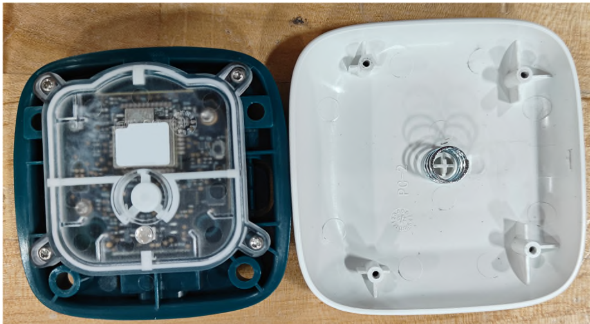
Figure 2 – Internal photo – Wall Button
