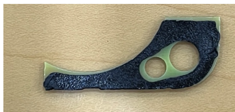
Figure 12 – SubGig PCB Antenna Back
