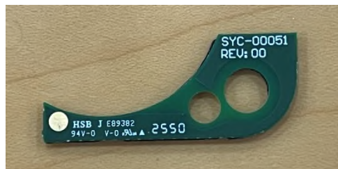
Figure 11 – SubGig PCB Antenna Front
