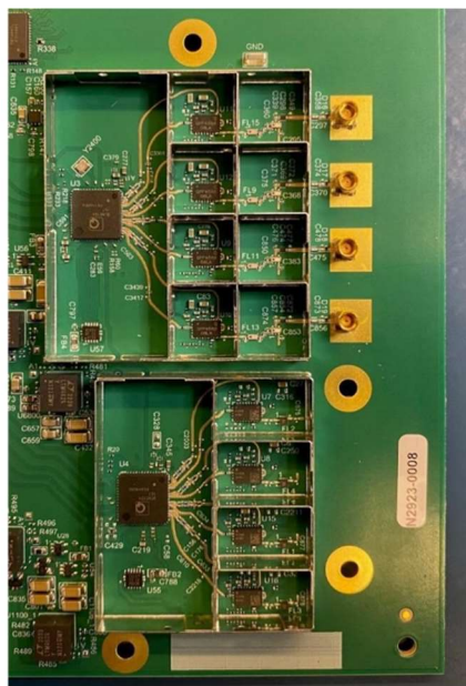
Figure 2-2: RF Front End Circuitry (Top – Left Side, Bottom – Right Side)
