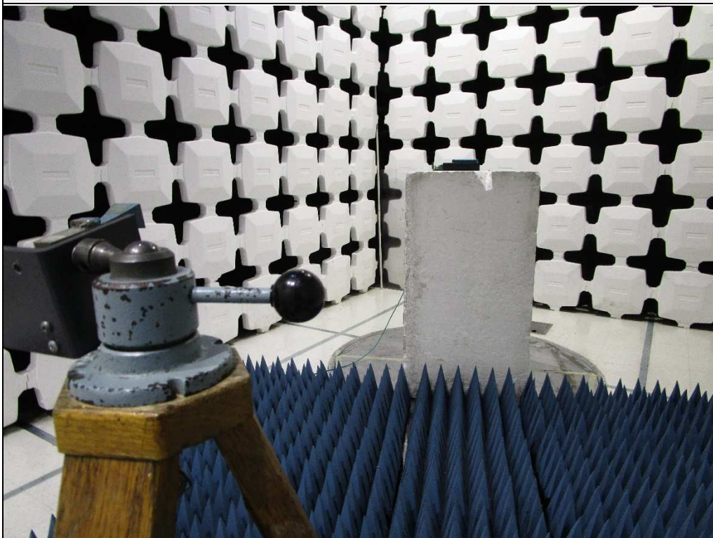
Test Setup for Spurious Radiated Emissions, Above 26.5GHz – Antenna Polarization Vertical
