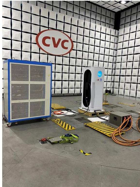
Setup photo of conducted emission (150KHz-30MHz)
