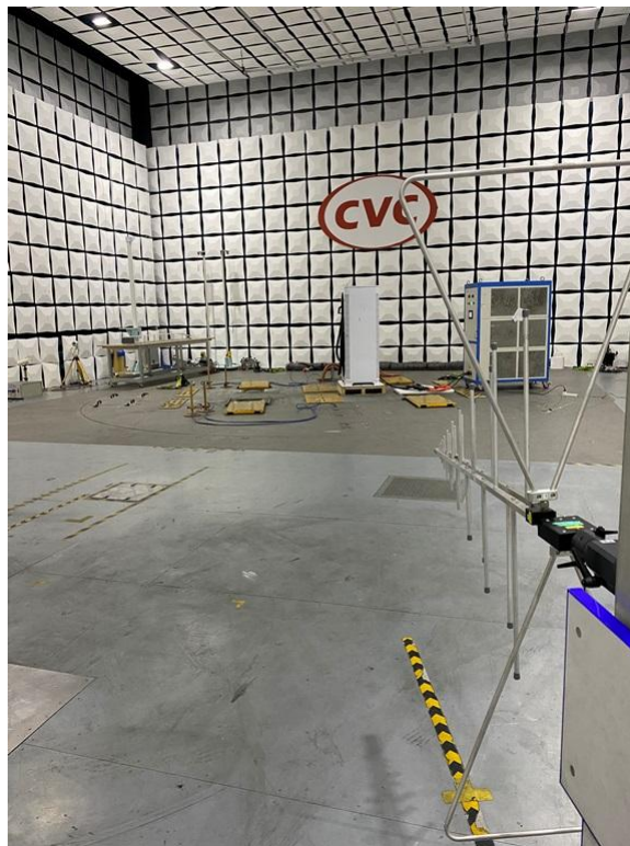
Setup photo of radiated emission (30MHz-1GHz)
