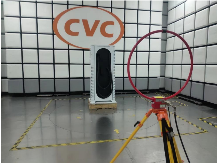
Setup photo of radiated emission (9KHz-30MHz)
