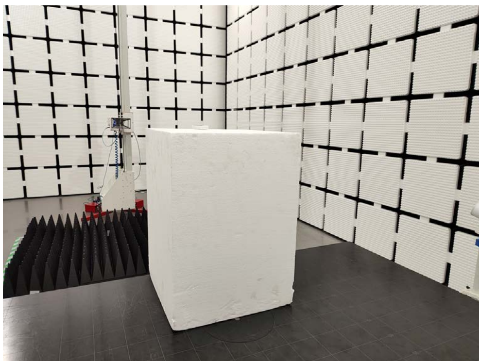
Spurious Radiation Emissions Test (>1G)
