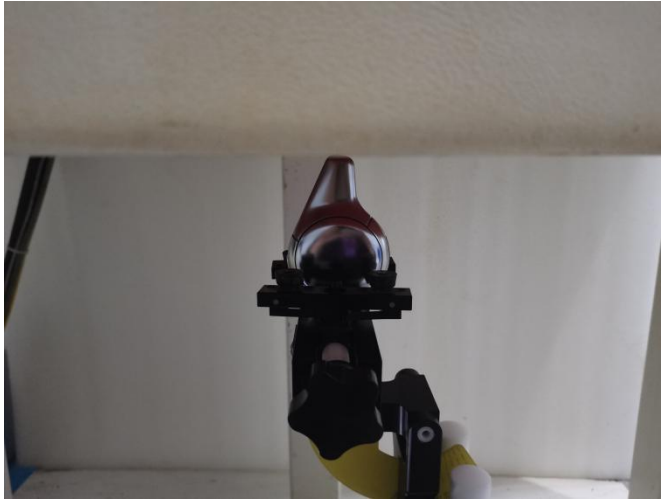
Fig-4.5 Top Side of EUT with 0 cm Gap (Body Mode)
