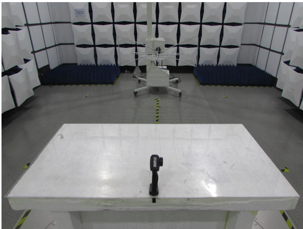
Radiated Emission Below 1GHz
