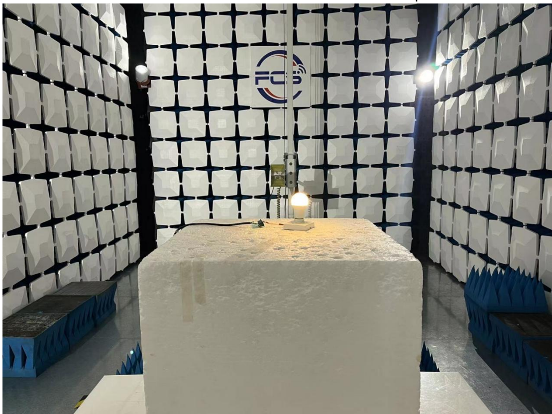
Above 1GHz for radiated emission test setup
