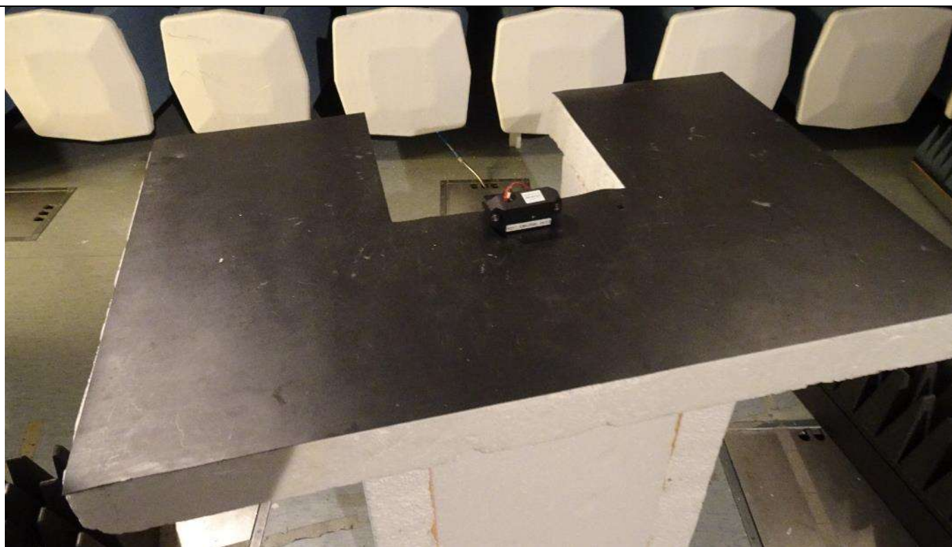
Picture 18, Radiated Spurious Emissions, EUT setup, RX 1 – 18 GHz, front view
