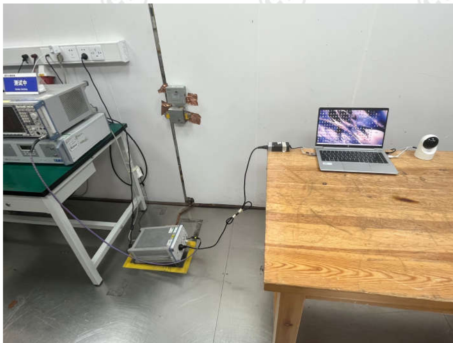
Conducted Emissions Test Setup
