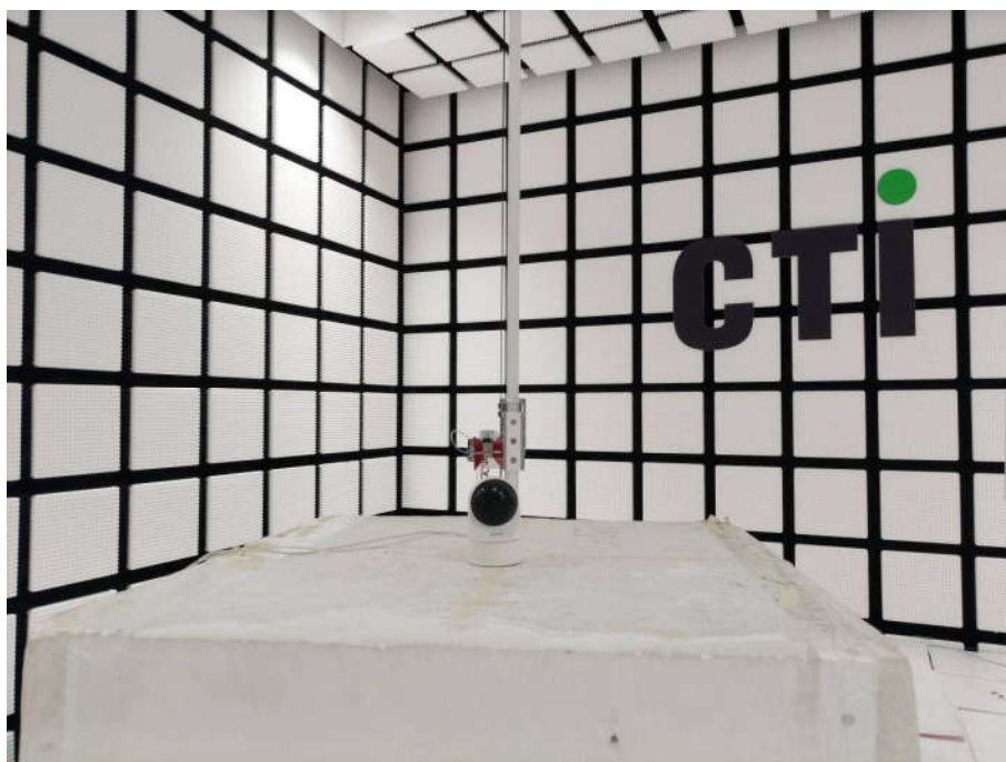
Radiated spurious emission Test Setup-2(Above 1GHz)
