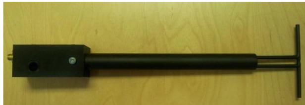
Figure 1 – MVG COMOSAR Validation Dipole
