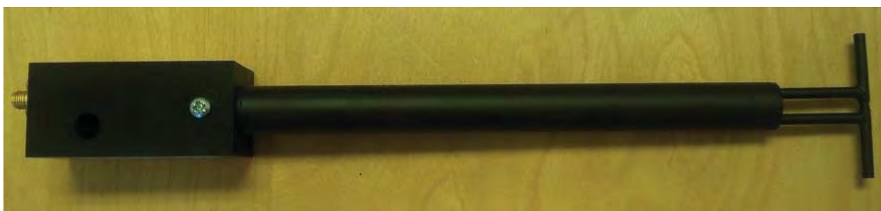
Figure 1 – MVG COMOSAR Validation Dipole
