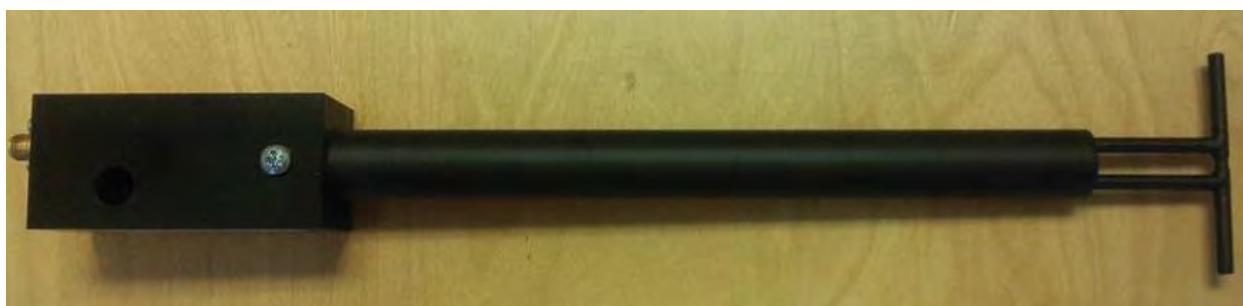
Figure 1 – MVG COMOSAR Validation Dipole
