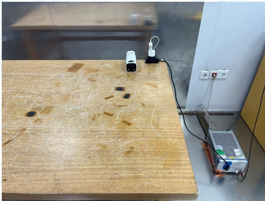
Photo of Setup for Radiated Emission (30MHz~1GHz)
