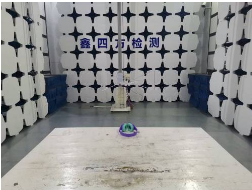
Photos of radiated emission test 30MHz – 1GHz
