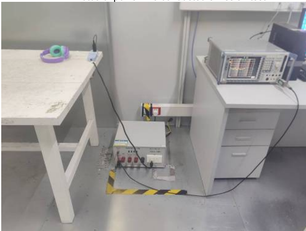
Photos of power line conducted emission test
