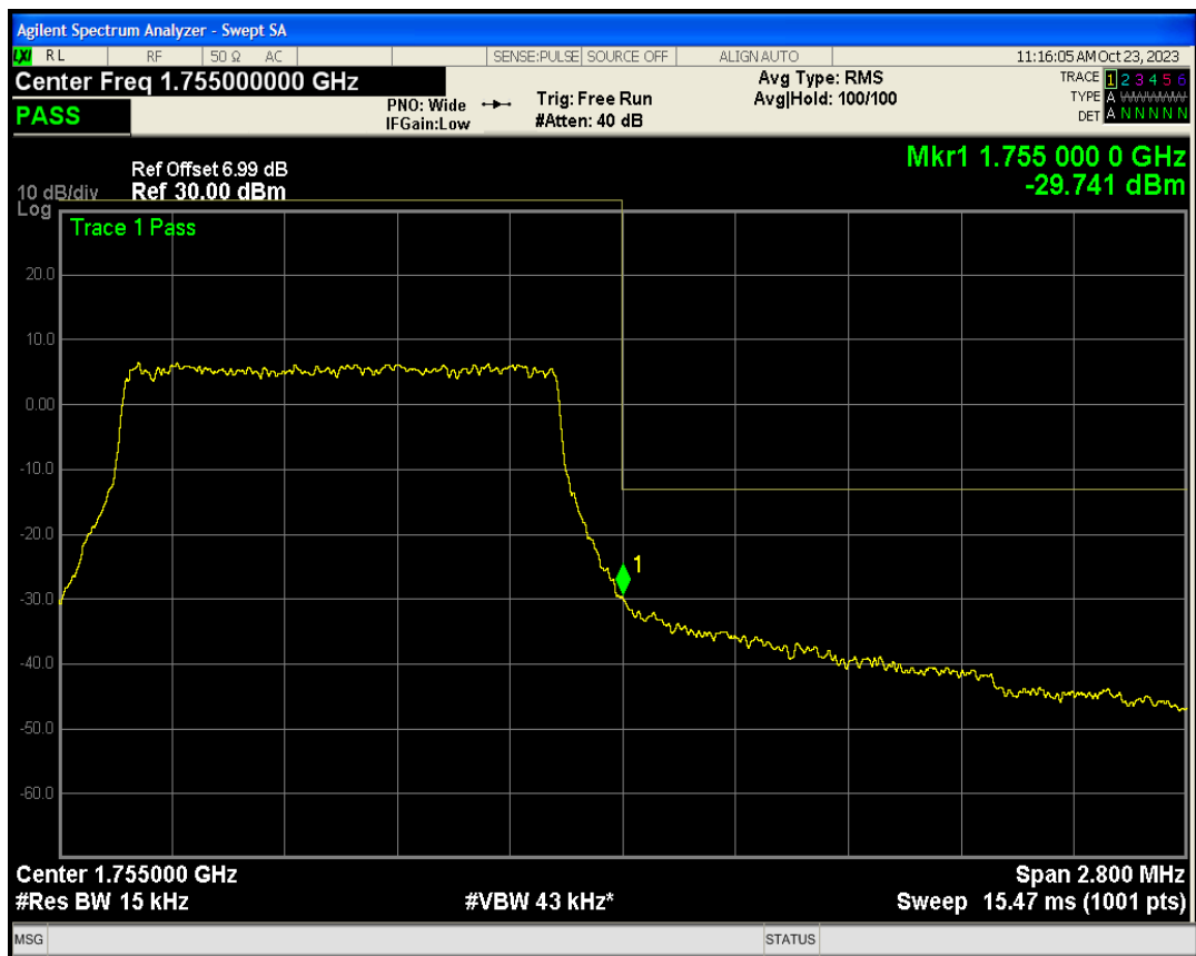
Band4 QAM16 BW=1.4MHz Channel=20393 RB Size=6 Position=#0
