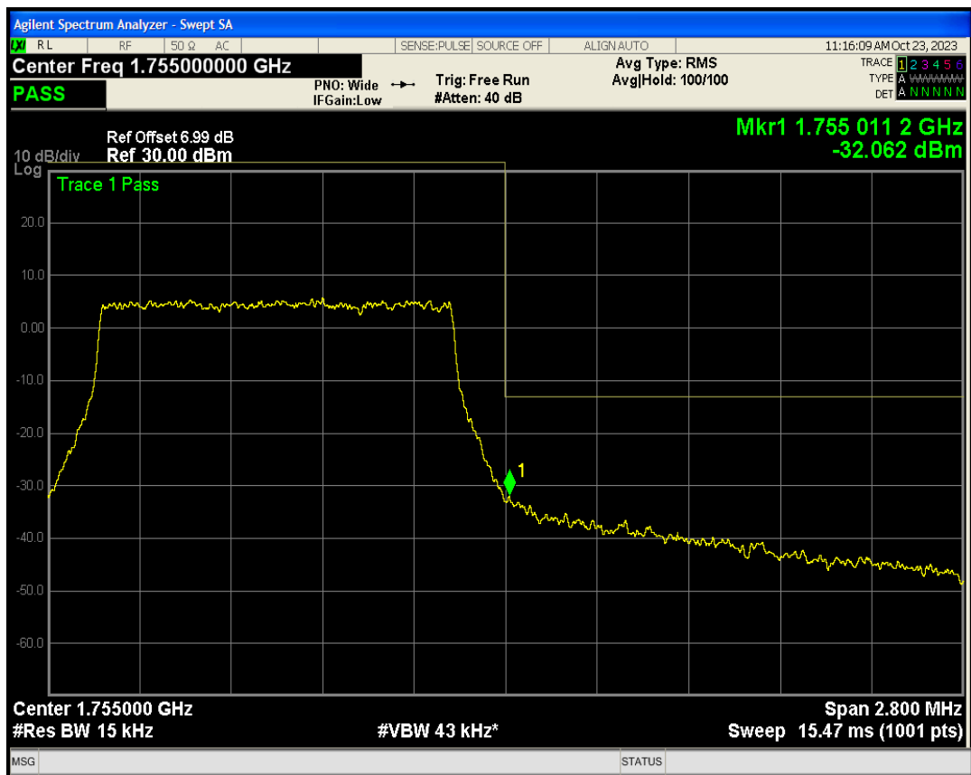
Band4 QPSK BW=3MHz Channel=19965 RB Size=15 Position=#0
