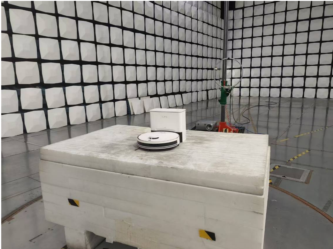
Radiated Emission 9k-30MHz Perpendicular View
