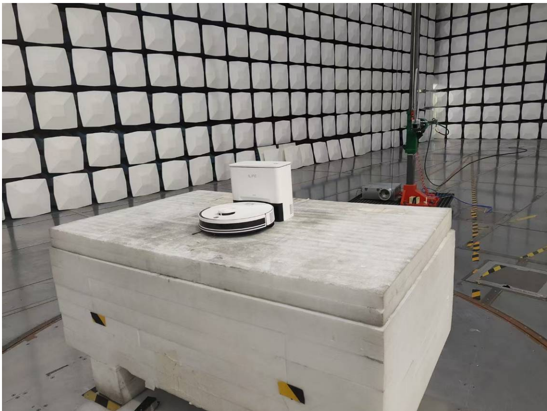
Radiated Emission 9k-30MHz Perpendicular View
