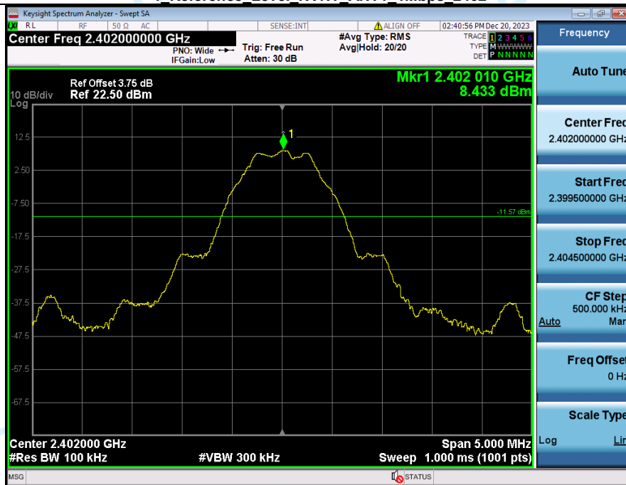
2 Spurious Emission NVNT ANT1 1Mbps 2402
