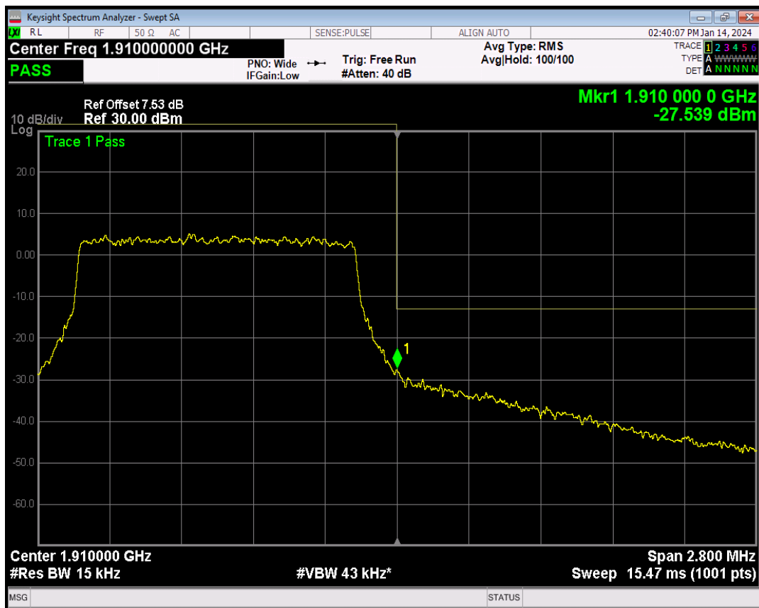
Band2 QPSK BW=3MHz Channel=18615 RB Size=1 Position=#0
