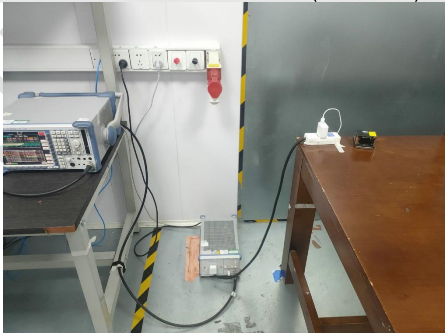
Conducted Emissions at Mains Terminals (150kHz-30MHz)
