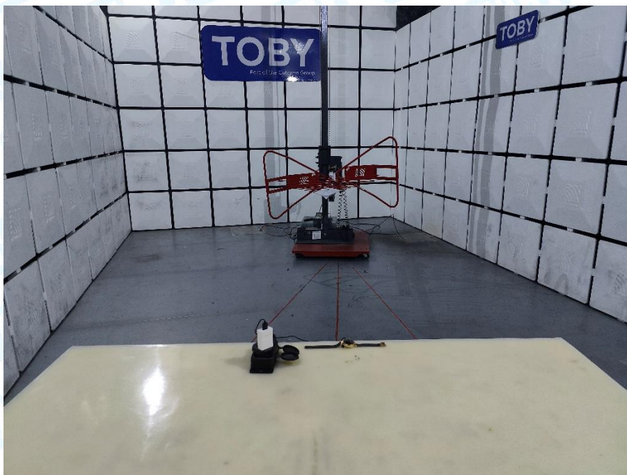
Photo of Setup for Radiated Emission (30MHz~1GHz)
