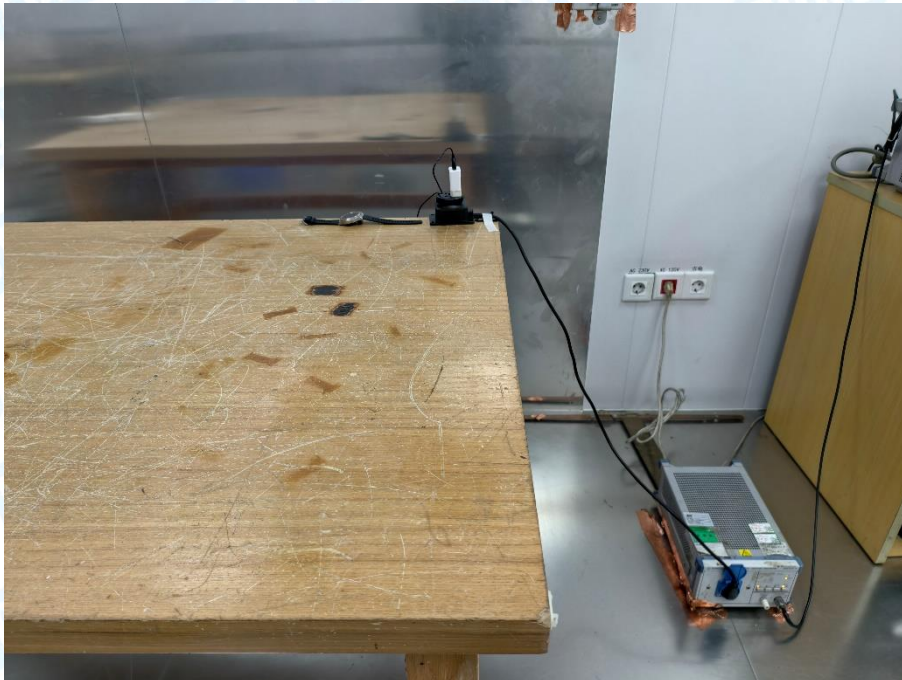
Photo of Setup for Radiated Emission (30MHz~1GHz)
