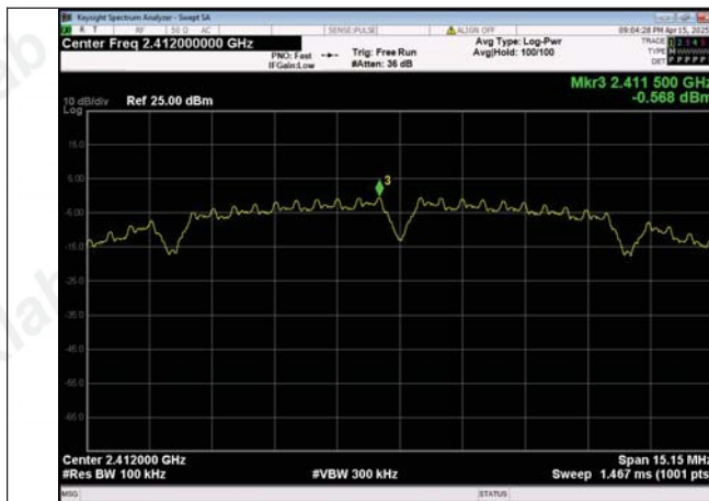
In-Band Reference Level IEEE 802.11b_Channel 1_20MHz
