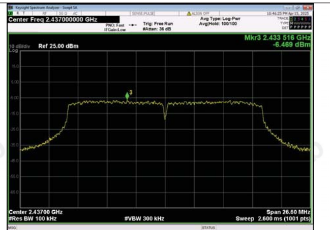
In-Band Reference Level IEEE 802.11n_Channel 6_20MHz
