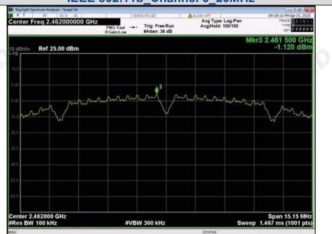
In-Band Reference Level IEEE 802.11b_Channel 11_20MHz
