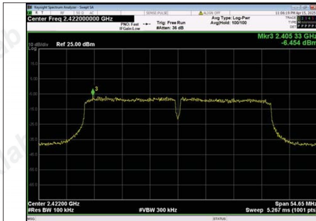
In-Band Reference Level IEEE 802.11n_Channel 3_40MHz
