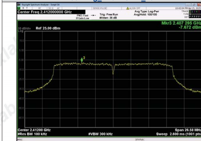
In-Band Reference Level IEEE 802.11n_Channel 1_20MHz
