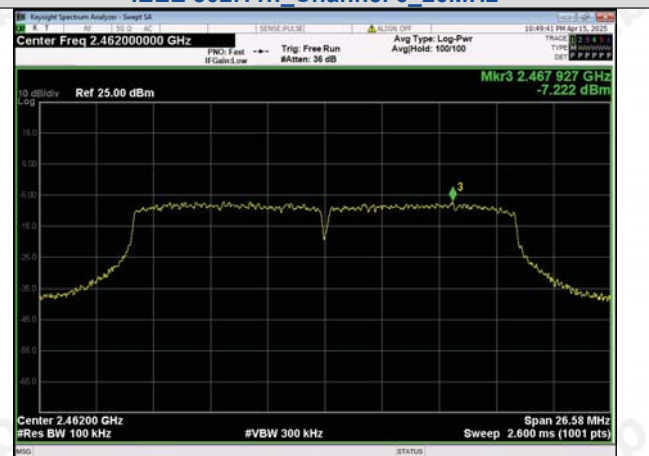
In-Band Reference Level IEEE 802.11n_Channel 11_20MHz
