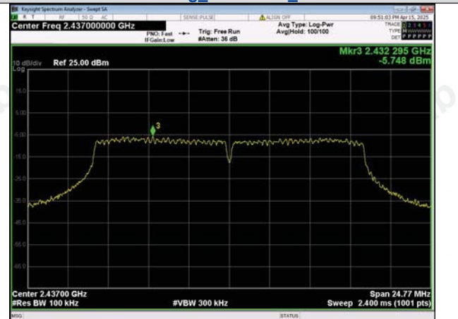
In-Band Reference Level IEEE 802.11g_Channel 6_20MHz
