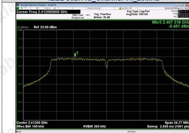
In-Band Reference Level IEEE 802.11g_Channel 1_20MHz
