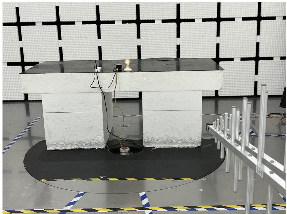
Radiation Emission Test Setup (30MHz to 1GHz)
