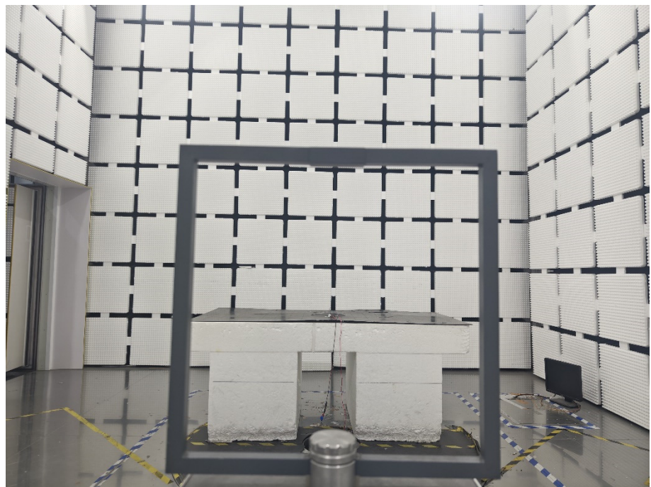
Radiation Emission Test Setup (Below 30MHz)
