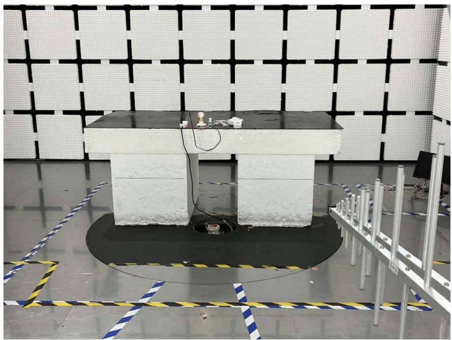
Radiation Emission Test Setup (30MHz to 1GHz)
