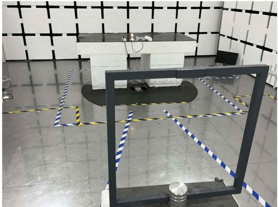
Radiation Emission Test Setup (Below 30MHz)
