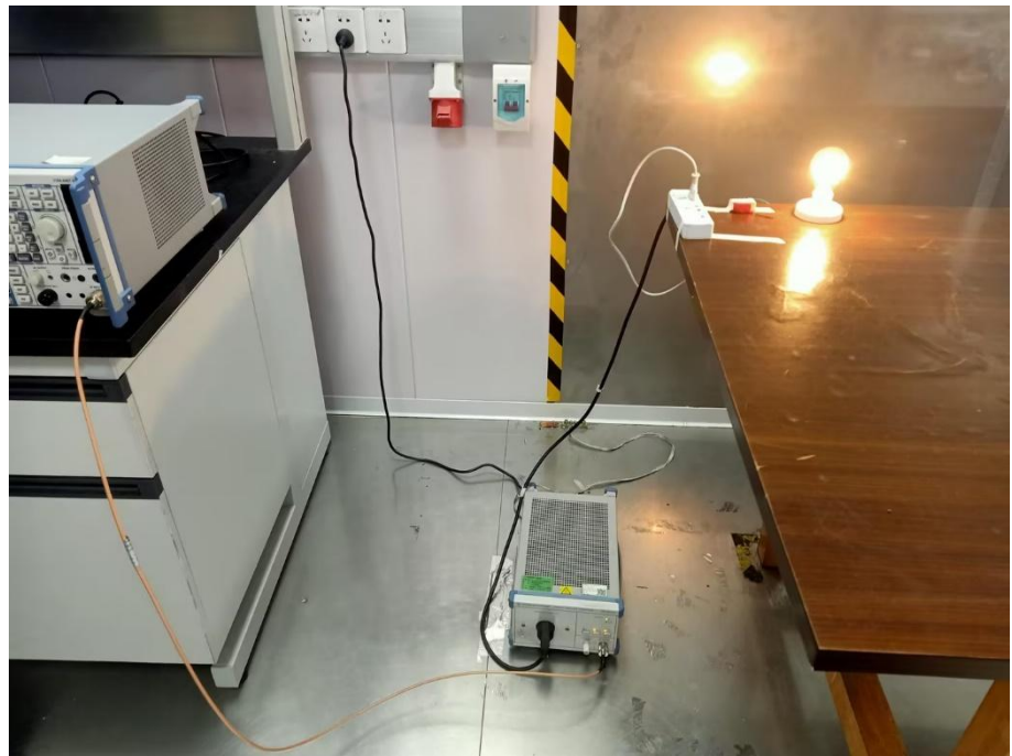
Conducted Emission Test Setup
