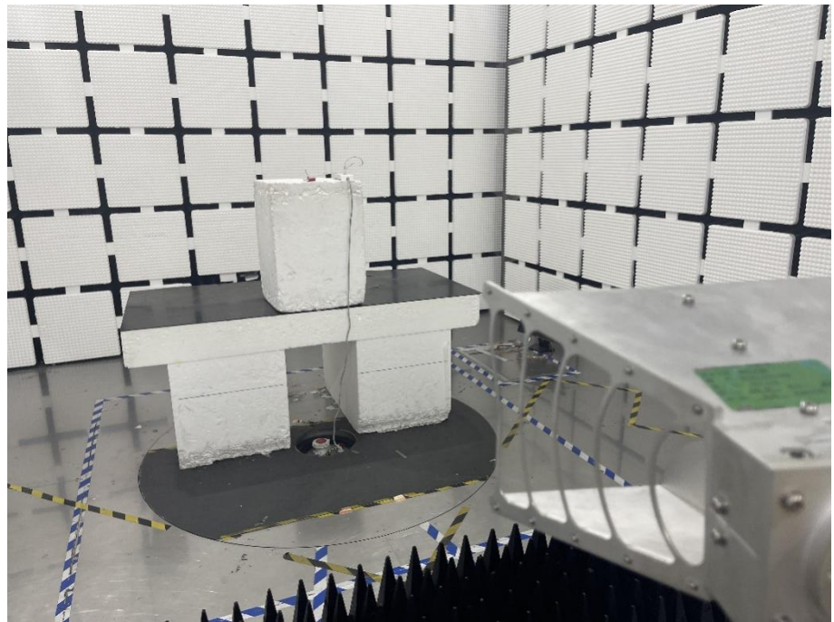
Radiation Emission Test Setup (1GHz to 18GHz)
