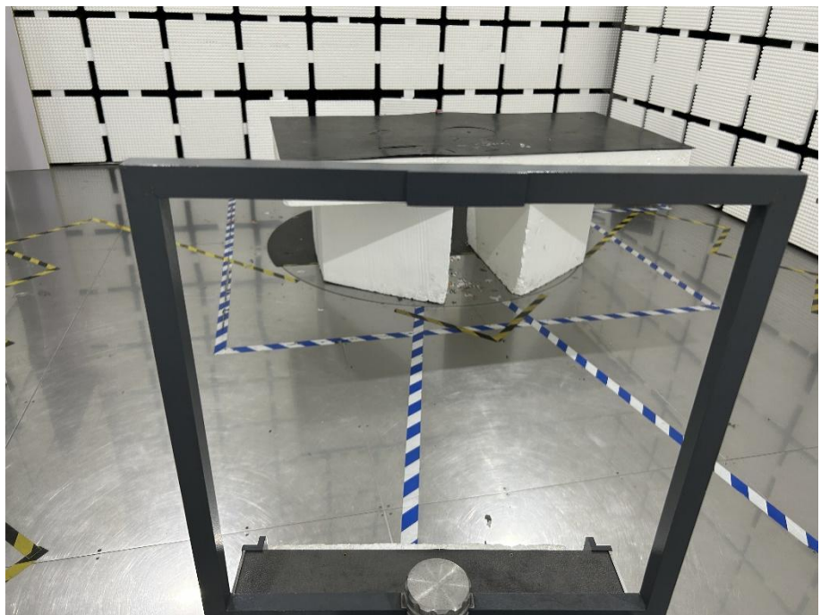
Radiation Emission Test Setup (Below 30MHz)
