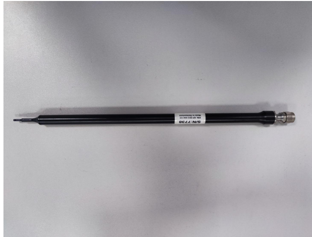
Figure 1-Speag COMOSAR Dosimetric E field Dipole
