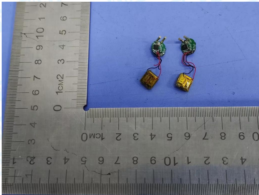
Photo 17 Appearance of PCB & Battery
