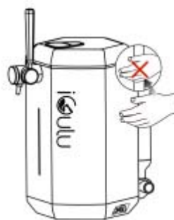
Wrong Way of Movement
