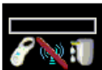
Figure 2-17: No radio communication to the alfapump®
