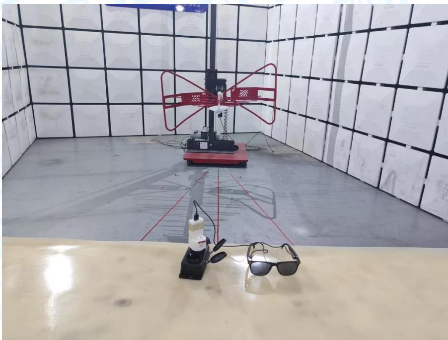
Photo of Setup for Radiated Emission (30MHz~1GHz)
