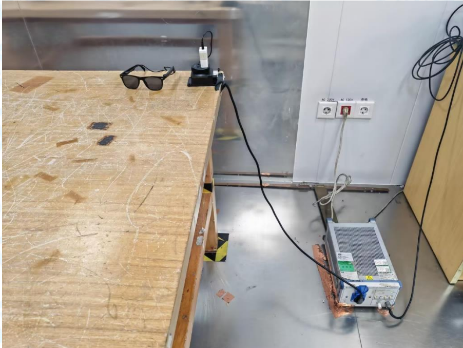
Photo of Setup for Radiated Emission (30MHz~1GHz)
