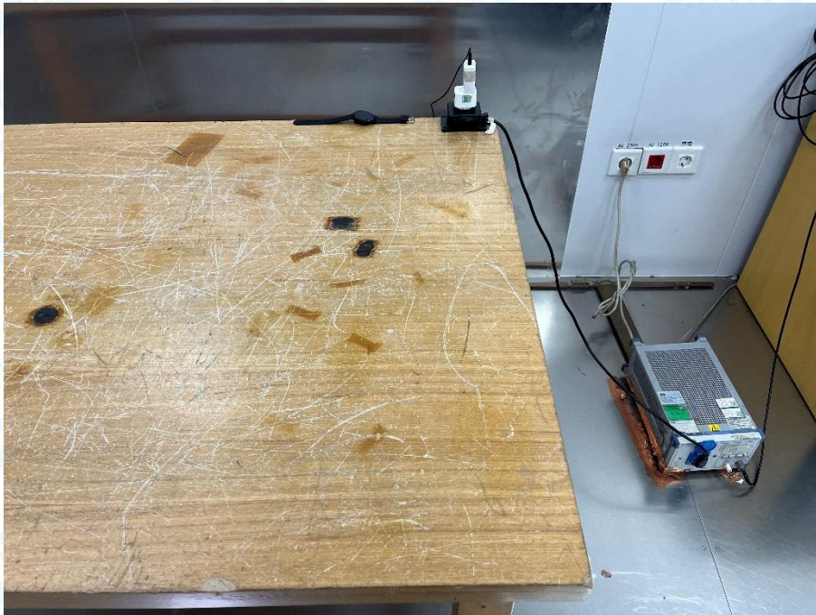
Photo of Setup for Radiated Emission (30MHz~1GHz)
