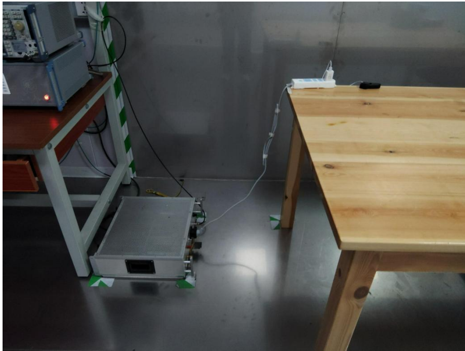
Conducted Emission at AC power line
