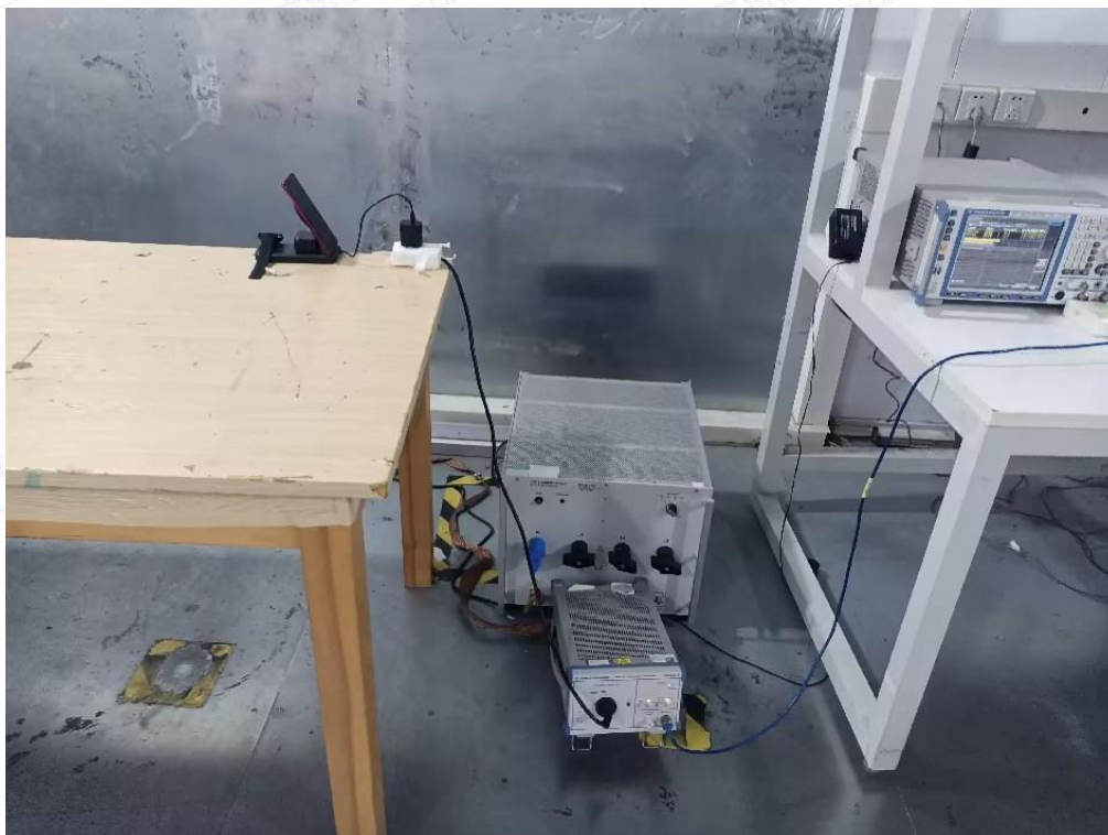
Conducted Emission-AC adapter charge mode
